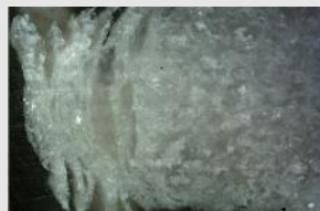
(above) Optical micrograph showing gradient porosity of SHS produced calcium phosphate with elongated pores on the left and small spherical pores on the right. Pores sizes range from 1 micron to 1000 microns.
